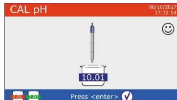
The actual measured value flashes on the display and subsequently, next to the beakers of pH 7.00 and pH 4.01, the icon of the beaker pH 10.01 appears, indicating that the instrument is calibrated in the alkaline field.
